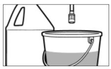
Step 2 Fill a container with Karcher detergent. Place the filter end of detergent suction tube into the container.
